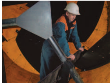
Drum mixer with our replaceable rubber or PU linings.
