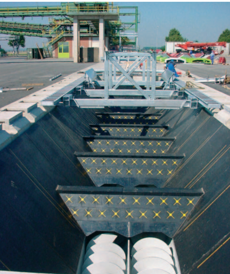
Feed chute at a sugar plant lined with Trellex SQ Modules and PP-XL wear plates.
