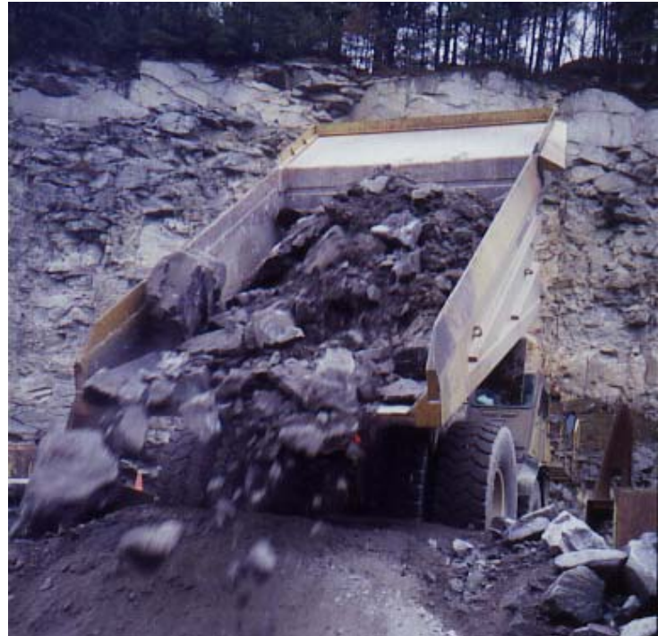
Truck type Cat lined with Trellex wear resistant elements type PP.
