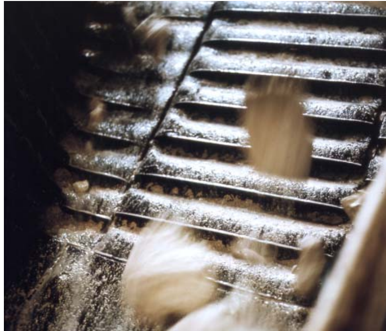
Trellex profiled Rubber Elements in chute.
